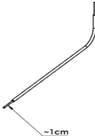
2. Find a non-magnetic box of about 2.5 to 4 cm height. Using some tape, fix the wires about 1.5 cm apart and with the tips of the wire about 3.5 cm from the edge of the box. Bend the part of the wires that are on the box upwards so that you can easily make connections to them. The exposed wire should be as horizontal. Measure the separation of the wires as accurately as you can.
