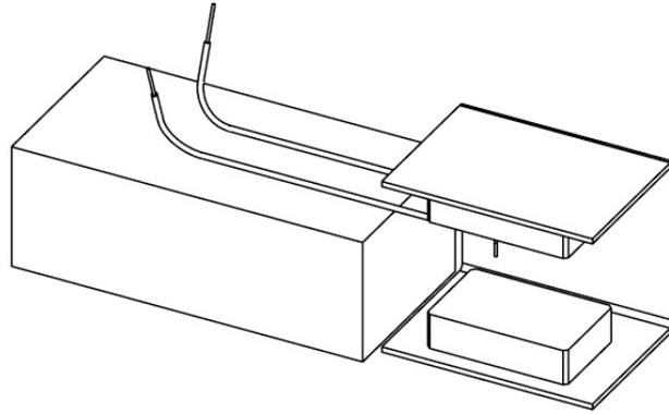
7. Briefly close the circuit. The bridge wire will move either towards the support and hit the insulated end of the wire or in the opposite direction and fall off. If it moves towards the support, reverse the direction of the magnetic field by turning the magnet assembly around. You want to orient the field so that the bridge wire falls off away from the assembly.
