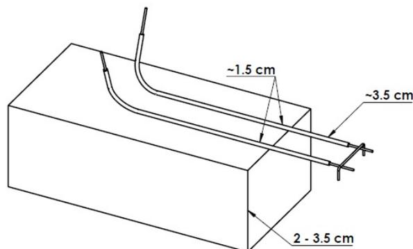
3. Cut a short length of wire of about 3 cm length and remove all the insulation from it. Measure the length of the wire as accurately as you can. Using a blade or emery paper, lightly clean it to remove any oxide that may have formed on its surface. Bend it in the
