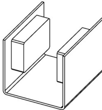
6. With the circuit open, place the magnet arrangement so that the magnetic field is in the vertical direction and centered around the bridge wire.
